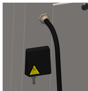
Figure 8: Hose connection for compressed air
